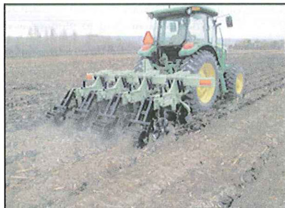
Strip tilling in fall 2014 at the Western Colorado Research Center at Fruita in a furrow-irrigated corn field that was burned to reduce residue to a manageable level. This approach reduced the number of field operations needed to prepare a high quality seedbed for planting in spring 2015.
